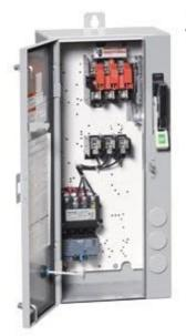
Non-reversing motor starter, Size 0, Three phase full voltage, Solidstate overload relay, OLRelay amp range 3-12a, 24Vdc coil, Combination type, 30Amp fusible disconnect 30 Amp /250V fuse clip, Enclosure NEMA type 4/12, Water/dust tight for outdoors, Standard width enclosure
