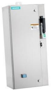
Non-reversing motor starter Size 0 Three phase full voltage Solidstate overload relay OLRelay amp range 3-12A Combination type 30Amp fusible disconnect 30Amp / 250V fuse clip Encl NEMA type 4X 316 S-steel Water/dust tight non-corrosive Standard width enclosure
