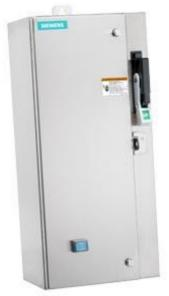
Non-reversing motor starter Size 0 Three phase full voltage Solidstate overload relay OLRelay amp range 3-12A Combination type 30Amp fusible disconnect 30 Amp /600V fuse clip Encl NEMA type 4X 316 S-steel Water/dust tight non-corrosive Standard width enclosure
