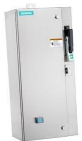
Non-reversing motor starter Size 0 Three phase full voltage Solidstate overload relay OLRelay amp range 3-12A 208VAC 60HZ coil Combination type 30Amp non-fusible disconnect Encl NEMA type 4X 316 S-steel Water/dust tight non-corrosive Standard width enclosure
