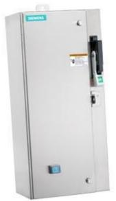
Non-reversing motor starter Size 0 Three phase full voltage Solidstate overload relay OLRelay amp range 3-12A Combination type 30Amp non-fusible disconnect Encl NEMA type 4X 316 S-steel Water/dust tight non-corrosive Standard width enclosure
