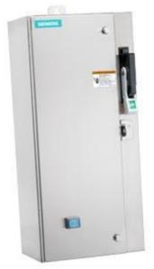
Non-reversing motor starter Size 0 Three phase full voltage Solidstate overload relay OLRelay amp range 3-12A 240VAC 50HZ / 277VAC 60HZ coil Combination type 30Amp fusible disconnect 30Amp / 250V fuse clip Encl NEMA type 4X 316 S-steel Water/dust tight non-corrosive Standard width enclosure
