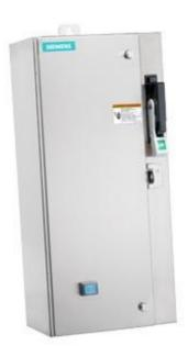
Non-reversing motor starter Size 0 Three phase full voltage Solidstate overload relay OLRelay amp range 3-12A 240VAC 50HZ / 277VAC 60HZ coil Combination type 30Amp non-fusible disconnect Encl NEMA type 4X 316 S-steel Water/dust tight non-corrosive Standard width enclosure
