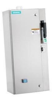
Non-reversing motor starter Size 0 Three phase full voltage Solidstate overload relay OLRelay amp range 3-12A 24Vdc coil Combination type 30Amp fusible disconnect 30 Amp /600V fuse clip Encl NEMA type 4X 316 S-steel Water/dust tight non-corrosive Standard width enclosure
