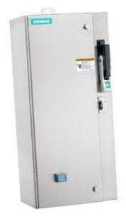
Non-reversing motor starter Size 0 Three phase full voltage Solidstate overload relay OLRelay amp range 3-12A 24Vdc coil Combination type 30Amp non-fusible disconnect Encl NEMA type 4X 316 S-steel Water/dust tight non-corrosive Standard width enclosure
