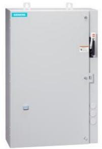
Non-reversing motor starter Size 0 Three phase full voltage Solidstate overload relay OLRelay amp range 5.5-22A 24Vdc coil Combination type 30Amp fusible disconnect 30Amp / 250V fuse clip Encl NEMA type 4X 304 S-steel Water/dust tight non-corrosive Extrawide enclosure
