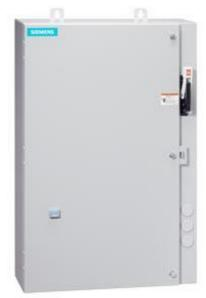
Non-reversing motor starter Size 0 Three phase full voltage Solidstate overload relay OLRelay amp range 5.5-22A 24Vdc coil Combination type 30Amp non-fusible disconnect Encl NEMA type 4X 304 S-steel Water/dust tight non-corrosive Extra-wide enclosure
