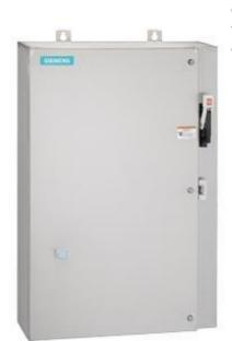
Non-reversing motor starter Size 0 Three phase full voltage Solidstate overload relay OLRelay amp range 5.5-22A 24VAC 50-60HZ coil Combination type 30Amp non-fusible disconnect Encl NEMA type 4X 316 S-steel Water/dust tight non-corrosive Extra-wide enclosure
