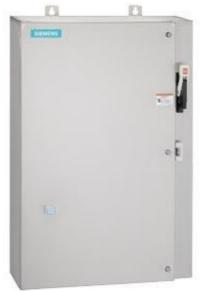
Non-reversing motor starter Size 0 Three phase full voltage Solidstate overload relay OLRelay amp range 5.5-22A 240VAC 50HZ / 277VAC 60HZ coil Combination type 30Amp non-fusible disconnect Encl NEMA type 4X 316 S-steel Water/dust tight non-corrosive Extrawide enclosure
