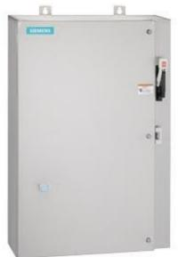
Non-reversing motor starter Size 0 Three phase full voltage Solidstate overload relay OLRelay amp range 5.5-22A 24Vdc coil Combination type 30Amp fusible disconnect 30Amp / 250V fuse clip Encl NEMA type 4X 316 S-steel Water/dust tight non-corrosive Extrawide enclosure
