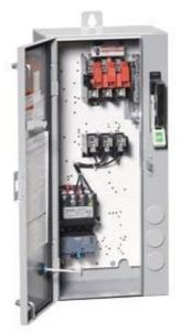
Non-reversing motor starter Size 0 Three phase full voltage Solidstate overload relay OLRelay amp range 5.5-22A 110-120/220-240VAC 60HZ coil Combination type 30Amp fusible disconnect 30Amp / 250V fuse clip Enclosure NEMA type 4/12 Water/dust tight weather proof Standard width enclosure
