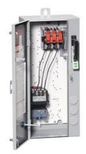
Non-reversing motor starter, Size 0, Three phase full voltage, Solidstate overload relay, OLRelay amp range 5.5-22a, 110V 50HZ / 120V 60HZ coil, Combination type, 30Amp non-fusible disconnect Enclosure NEMA type 4/12, Water/dust tight for outdoors, Standard width enclosure
