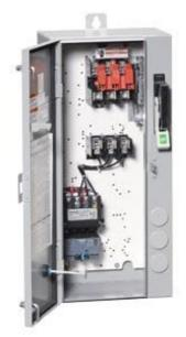
Non-reversing motor starter Size 0 Three phase full voltage Solidstate overload relay OLRelay amp range 5.5-22A 24Vdc coil Combination type 30Amp fusible disconnect 30Amp / 250V fuse clip Enclosure NEMA type 4/12 Water/dust tight weather proof Standard width enclosure
