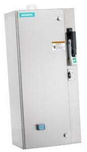
Non-reversing motor starter Size 0 Three phase full voltage Solidstate overload relay OLRelay amp range 5.5-22A Combination type 30Amp fusible disconnect 30Amp / 250V fuse clip Encl NEMA type 4X 316 S-steel Water/dust tight non-corrosive Standard width enclosure
