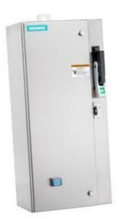
Non-reversing motor starter Size 0 Three phase full voltage Solidstate overload relay OLRelay amp range 5.5-22A 208VAC 60HZ coil Combination type 30Amp fusible disconnect 30Amp / 250V fuse clip Encl NEMA type 4X 316 S-steel Water/dust tight non-corrosive Standard width enclosure
