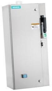
Non-reversing motor starter, Size 0, Three phase full voltage, Solid-state overload relay, OLRelay amp range 5.5-22a, 110V 50HZ / 120V 60HZ coil, Combination type, 30Amp fusible disconnect 30 Amp /250V fuse clip, Encl NEMA type 4X 316 S-steel Water/dust tight noncorrosive, Standard width enclosure
