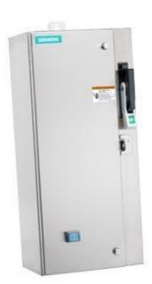
Non-reversing motor starter, Size 0, Three phase full voltage, Solidstate overload relay, OLRelay amp range 5.5-22a, 110V 50HZ / 120V 60HZ coil, Combination type, 30Amp non-fusible disconnect Encl NEMA type 4X 316 S-steel Water/dust tight noncorrosive, Standard width enclosure
