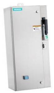
Non-reversing motor starter Size 0 Three phase full voltage Solidstate overload relay OLRelay amp range 5.5-22A Combination type 30Amp non-fusible disconnect Encl NEMA type 4X 316 S-steel Water/dust tight non-corrosive Standard width enclosure
