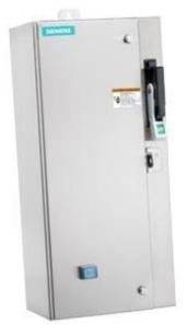
Non-reversing motor starter Size 0 Three phase full voltage Solidstate overload relay OLRelay amp range 5.5-22A 24VAC 50-60HZ coil Combination type 30Amp fusible disconnect 30Amp / 250V fuse clip Encl NEMA type 4X 316 S-steel Water/dust tight non-corrosive Standard width enclosure
