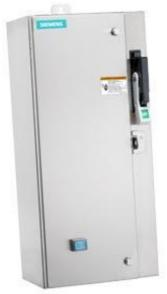
Non-reversing motor starter Size 0 Three phase full voltage Solidstate overload relay OLRelay amp range 5.5-22A 240VAC 50HZ / 277VAC 60HZ coil Combination type 30Amp non-fusible disconnect Encl NEMA type 4X 316 S-steel Water/dust tight non-corrosive Standard width enclosure
