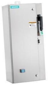
Non-reversing motor starter Size 0 Three phase full voltage Solidstate overload relay OLRelay amp range 5.5-22A 24Vdc coil Combination type 30Amp fusible disconnect 30Amp / 250V fuse clip Encl NEMA type 4X 316 S-steel Water/dust tight non-corrosive Standard width enclosure
