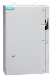
Non-reversing motor starter Size 1 Three phase full voltage Amb compensate bimetal OLrelay Contactor amp rating 27Amp Combination type 30Amp non-fusible disconnect Enclosure NEMA type 4/12 Water/dust tight weather proof Extra-wide enclosure
