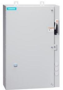
Non-reversing motor starter Size 1 Three phase full voltage Amb compensate bimetal OLrelay Contactor amp rating 27Amp 550/575-600 50/60HZ coil Combination type 30Amp fusible disconnect 30Amp / 250V fuse clip Enclosure NEMA type 4/12 Water/dust tight weather proof Extra-wide enclosure
