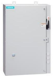
Non-reversing motor starter Size 1 Three phase full voltage Amb compensate bimetal OLrelay Contactor amp rating 27Amp 24VAC 50-60HZ coil Combination type 30Amp fusible disconnect 30Amp / 250V fuse clip Enclosure NEMA type 4/12 Water/dust tight weather proof Extra-wide enclosure
