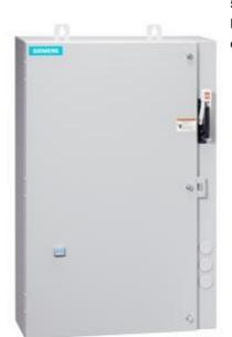
Non-reversing motor starter Size 1 Three phase full voltage Amb compensate bimetal OLrelay Contactor amp rating 27Amp 24VAC 50-60HZ coil Combination type 30Amp non-fusible disconnect Enclosure NEMA type 4/12 Water/dust tight weather proof Extra-wide enclosure
