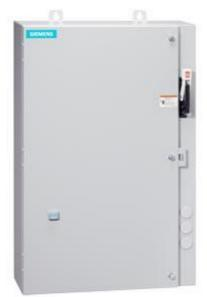
Non-reversing motor starter Size 1 Three phase full voltage Amb compensate bimetal OLrelay Contactor amp rating 27Amp 240VAC 50HZ / 277VAC 60HZ coil Combination type 30Amp fusible disconnect 30Amp / 250V fuse clip Enclosure NEMA type 4/12 Water/dust tight weather proof Extra-wide enclosure
