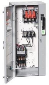
Non-reversing motor starter Size 1 Three phase full voltage Amb compensate bimetal OLrelay Contactor amp rating 27Amp 110VAC 50HZ / 120VAC 60HZ coil Combination type 30Amp fusible disconnect 30 Amp /600V fuse clip Enclosure NEMA type 1 Indoor general purpose use Standard width enclosure
