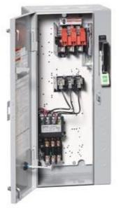
Non-reversing motor starter Size 1 Three phase full voltage Amb compensate bimetal OLrelay Contactor amp rating 27Amp 380-440/440-480V 50/60HZ coil Combination type 30Amp fusible disconnect 30Amp / 250V fuse clip Enclosure NEMA type 1 Indoor general purpose use Standard width enclosure
