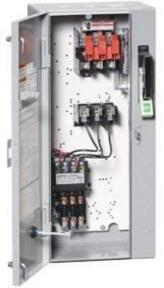
Non-reversing motor starter Size 1 Three phase full voltage Amb compensate bimetal OLrelay Contactor amp rating 27Amp 24Vdc coil Combination type 30Amp fusible disconnect 30 Amp /600V fuse clip Enclosure NEMA type 1 Indoor general purpose use Standard width enclosure
