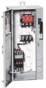
Non-reversing motor starter Size 1 Three phase full voltage Amb compensate bimetal OLrelay Contactor amp rating 27Amp Combination type 30Amp fusible disconnect 30Amp / 250V fuse clip Enclosure NEMA type 4/12 Water/dust tight weather proof Standard width enclosure
