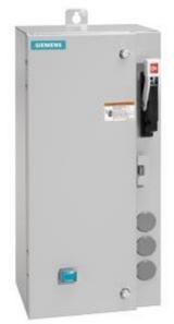
Non-reversing motor starter Size 1 Three phase full voltage Amb compensate bimetal OLrelay Contactor amp rating 27Amp 220-240/440-480VAC 60HZ coil Combination type 30Amp non-fusible disconnect Enclosure NEMA type 4/12 Water/dust tight weather proof Standard width enclosure
