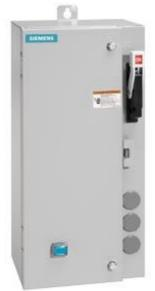
Non-reversing motor starter, Size 1, Three phase full voltage, Amb compensate bimetal OLrelay Contactor amp rating 27Amp 220 240/440 480VAC 60HZ coil, Combination type, 30Amp non-fusible disconnect Enclosure NEMA type 4/12, Water/dust tight for outdoors, Standard width enclosure
