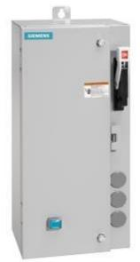
Non-reversing motor starter Size 1 Three phase full voltage Amb compensate bimetal OLrelay Contactor amp rating 27Amp 208VAC 60HZ coil Combination type 30Amp non-fusible disconnect Enclosure NEMA type 4/12 Water/dust tight weather proof Standard width enclosure
