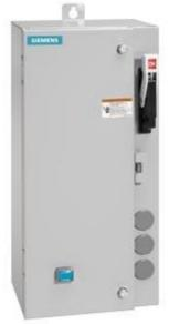
Non-reversing motor starter Size 1 Three phase full voltage Amb compensate bimetal OLrelay Contactor amp rating 27Amp 550/575-600 50/60HZ coil Combination type 30Amp non-fusible disconnect Enclosure NEMA type 4/12 Water/dust tight weather proof Standard width enclosure
