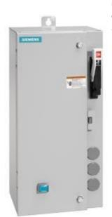
Non-reversing motor starter, Size 1, Three phase full voltage, Amb compensate bimetal OLrelay Contactor amp rating 27Amp 110V 50HZ / 120V 60HZ coil, Combination type, 30Amp non-fusible disconnect Enclosure NEMA type 4/12, Water/dust tight for outdoors, Standard width enclosure
