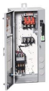
Non-reversing motor starter Size 1 Three phase full voltage Amb compensate bimetal OLrelay Contactor amp rating 27Amp Combination type 30Amp fusible disconnect 30Amp / 250V fuse clip Enclosure NEMA type 4/12 Water/dust tight weather proof Standard width enclosure
