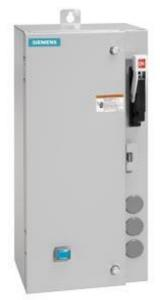
Non-reversing motor starter Size 1 Three phase full voltage Amb compensate bimetal OLrelay Contactor amp rating 27Amp 190-220/220-240V 50/60HZ coil Combination type 30Amp non-fusible disconnect Enclosure NEMA type 4/12 Water/dust tight weather proof Standard width enclosure
