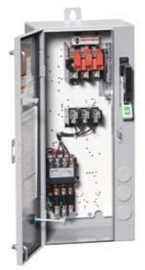
Non-reversing motor starter Size 1 Three phase full voltage Amb compensate bimetal OLrelay Contactor amp rating 27Amp 24VAC 50-60HZ coil Combination type 30Amp fusible disconnect 30Amp / 250V fuse clip Enclosure NEMA type 4/12 Water/dust tight weather proof Standard width enclosure
