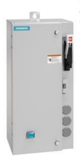
Non-reversing motor starter Size 1 Three phase full voltage Amb compensate bimetal OLrelay Contactor amp rating 27Amp 240VAC 50HZ / 277VAC 60HZ coil Combination type 30Amp non-fusible disconnect Enclosure NEMA type 4/12 Water/dust tight weather proof Standard width enclosure
