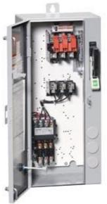
Non-reversing motor starter Size 1 Three phase full voltage Amb compensate bimetal OLrelay Contactor amp rating 27Amp 24Vdc coil Combination type 30Amp fusible disconnect 30 Amp /600V fuse clip Enclosure NEMA type 4/12 Water/dust tight weather proof Standard width enclosure
