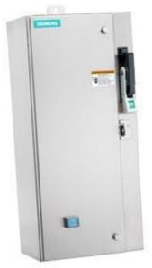
Non-reversing motor starter Size 1 Three phase full voltage Amb compensate bimetal OLrelay Contactor amp rating 27Amp Combination type 30Amp fusible disconnect 30Amp / 250V fuse clip Encl NEMA type 4X 304 S-steel Water/dust tight non-corrosive Standard width enclosure
