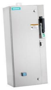
Non-reversing motor starter Size 1 Three phase full voltage Amb compensate bimetal OLrelay Contactor amp rating 27Amp 220-240/440-480VAC 60HZ coil Combination type 60Amp fusible disconnect 60Amp / 250V fuse clip Encl NEMA type 4X 304 S-steel Water/dust tight non-corrosive Standard width enclosure
