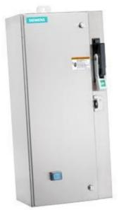
Non-reversing motor starter Size 1 Three phase full voltage Amb compensate bimetal OLrelay Contactor amp rating 27Amp 208VAC 60HZ coil Combination type 30Amp fusible disconnect 30 Amp /600V fuse clip Encl NEMA type 4X 304 S-steel Water/dust tight non-corrosive Standard width enclosure
