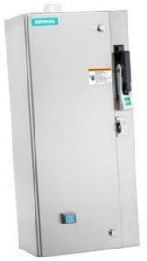
Non-reversing motor starter Size 1 Three phase full voltage Amb compensate bimetal OLrelay Contactor amp rating 27Amp 208VAC 60HZ coil Combination type 60Amp fusible disconnect 60Amp / 250V fuse clip Encl NEMA type 4X 304 S-steel Water/dust tight non-corrosive Standard width enclosure
