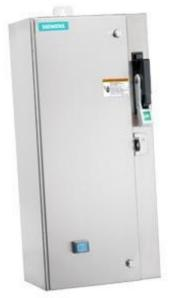
Non-reversing motor starter Size 1 Three phase full voltage Amb compensate bimetal OLrelay Contactor amp rating 27Amp 110VAC 50HZ / 120VAC 60HZ coil Combination type 30Amp fusible disconnect 30 Amp /600V fuse clip Encl NEMA type 4X 304 S-steel Water/dust tight non-corrosive Standard width enclosure
