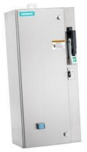
Non-reversing motor starter Size 1 Three phase full voltage Amb compensate bimetal OLrelay Contactor amp rating 27Amp 190-220/220-240V 50/60HZ coil Combination type 30Amp fusible disconnect 30 Amp /600V fuse clip Encl NEMA type 4X 304 S-steel Water/dust tight non-corrosive Standard width enclosure
